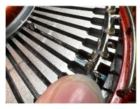
machine, ensure the Tappet switch is moved to the IN WORK position. All Ribber needles whenever added to a CSM are ALWAYS added with their latch open and the stitch in the needle not behind the latch.
