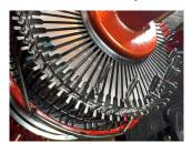
15) The first thing we need to do is take each Ribber needle while holding its stitch and place each Ribber needle upside down into its aligned cylinder slot. This will hold the stitch and clear the needle from the Ribber dial. Once all are moved remove the Ribber setup from the machine. Once the Ribber is lifted out easily put it safely aside and now to finish the Ribber Rest step where using your stitch tool gently lift the cylinder spring to gain access easily to the upside Ribber needles,
