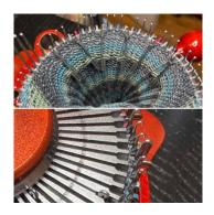
note there with be more tension than normal due to the loaded Ribber needles so for this row ensure to watch the knitting and give needed pull down on that first row with the added tension the knitting might not sit correctly low as
