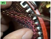
the yarn tail (next stitch bar on the same row) is our target first bar to hang on the cylinder. Now looking at the cylinder we note that the first slot after the 3 o'clock r
